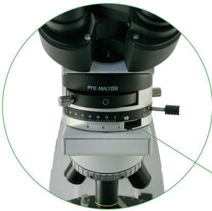
The Intermediate tube houses the Bertrand lens, analyzer, and slot for compensators: Gypsum 1gypsum 1 $\lambda$  plate, Mica 1/4  $\lambda$  plate, and Quartz wedge.
