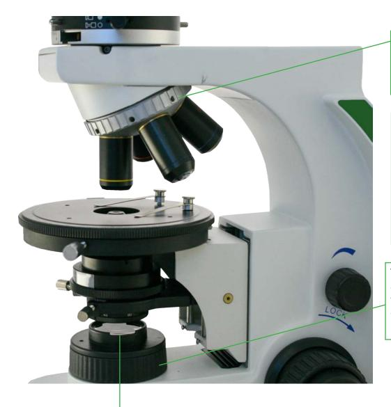
Each objective is centered by inserting the included centering screws into the objective centering holes.
