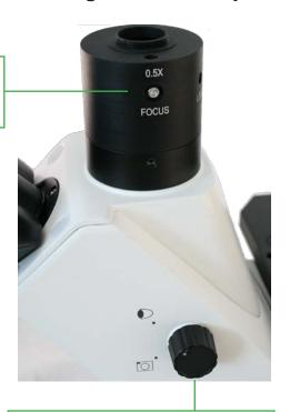
Direct light to the camera or the eyepieces with the turn of a knob.
