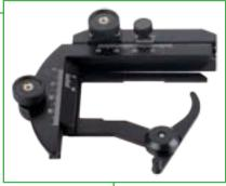
Attachable professional measuring mechanical stage provides more control over samples. Stage provides moving range of 30mm x 40mm with high precision micrometer reading 0.01mm increments.
